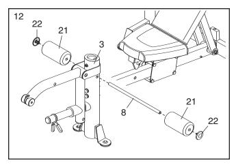
13. Insert the two Short Pad Tubes (15) into the Leg Lever (11). Slide two Foam Pads (21) onto each Short Pad Tube. Then, press a Pad Cap (22) into each Foam Pad.
